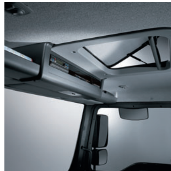
Storage compartment above windscreen and roof skylight in C cab.
