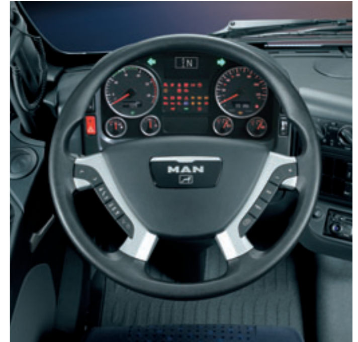
Multifunction steering wheel with controls for MAN radio and cruise control etc.
