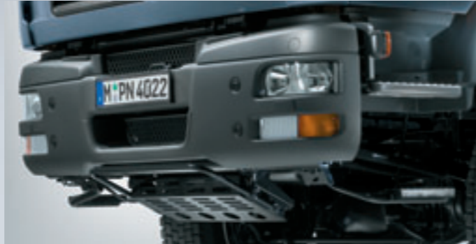
Strong steel bumper with the same appearance as the standard synthetic bumper.
