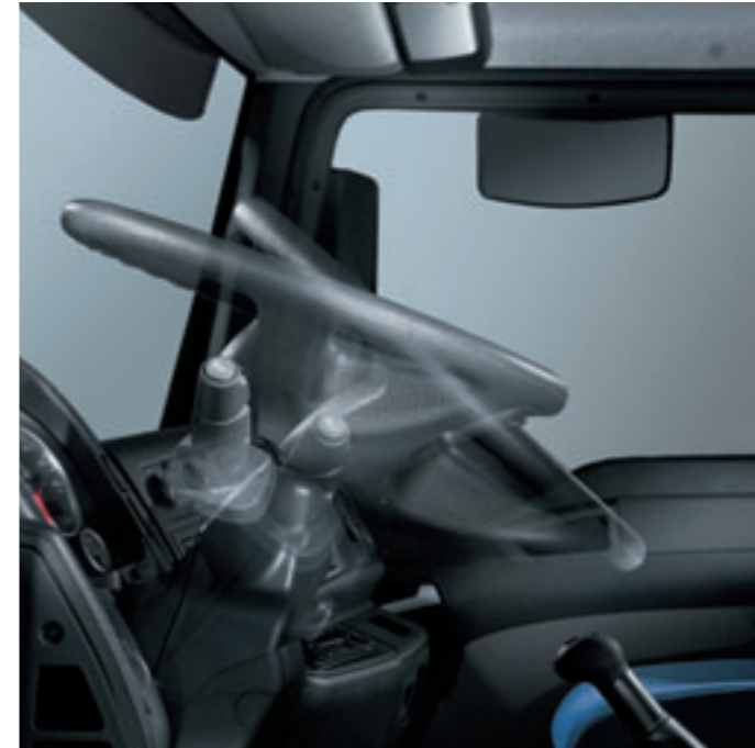
Pressing a footwell knob allows the steering wheel to be adjusted steplessly in height and angle.
